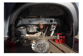
The reservoir should be mounted towards the top and pointing towards the front of the vehicle.
