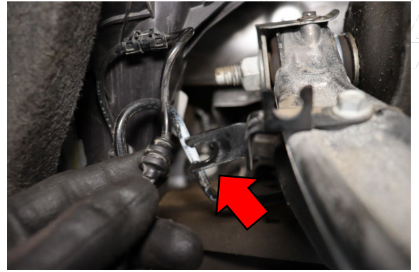
Step 2: Start by removing the wheel speed sensor from the bracket located on the upper control arm.
