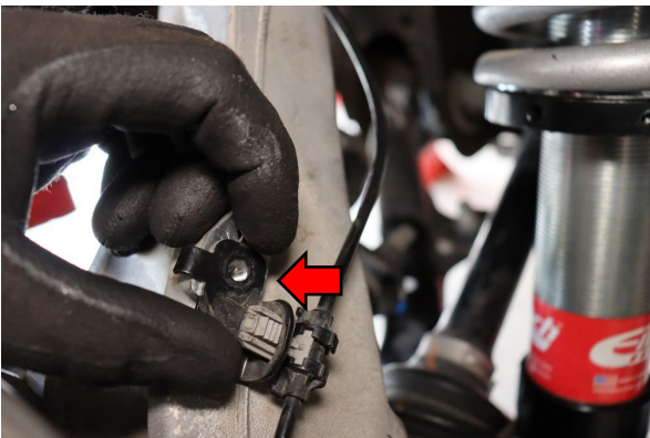
Step 17: Reinstall the bracket for the wheel speed sensor into the steering knuckle using a 10mm bolt.
