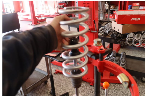
Install the Eibach tender spring.
