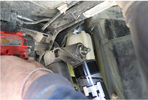
Loosen and remove the upper shock bolt.
