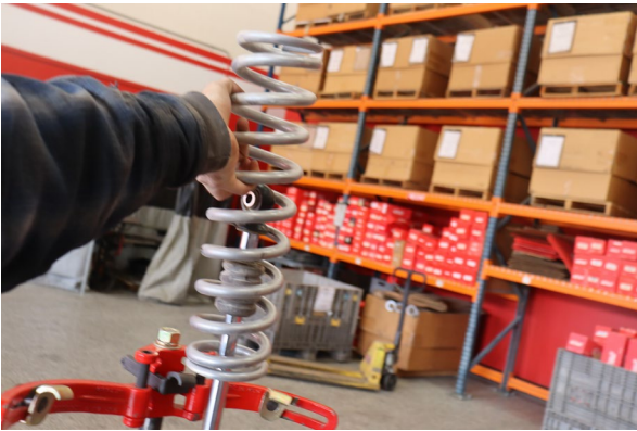
Install the Eibach main spring.
