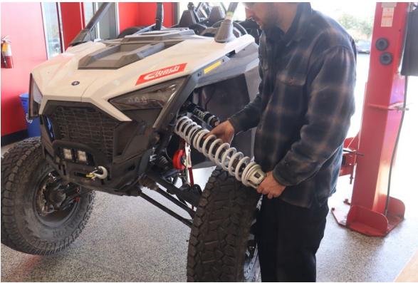
Remove the front shock.
