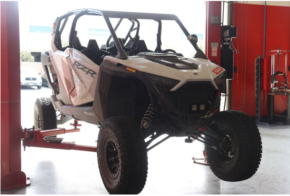
Begin by jacking up and safely supporting the front of the vehicle.
