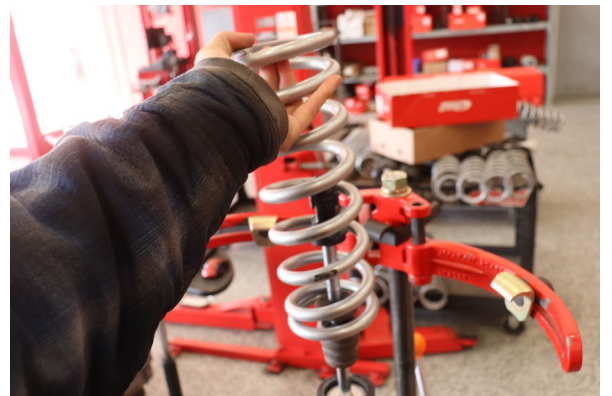
Install the Eibach main spring.
