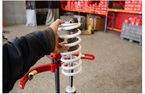
Remove the OE tender spring.
