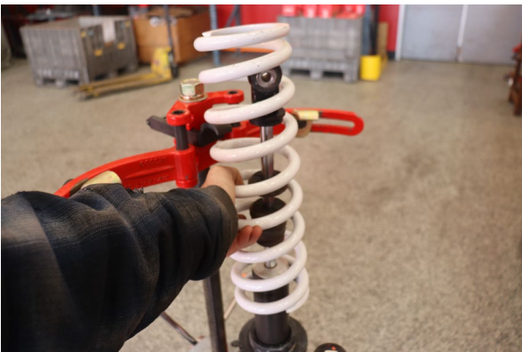
Remove the OE main spring.
