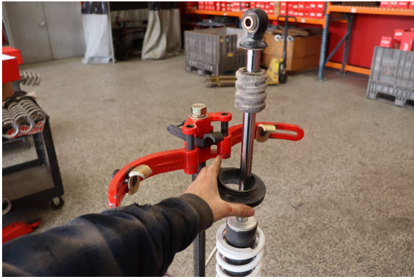
Remove the OE slider.
