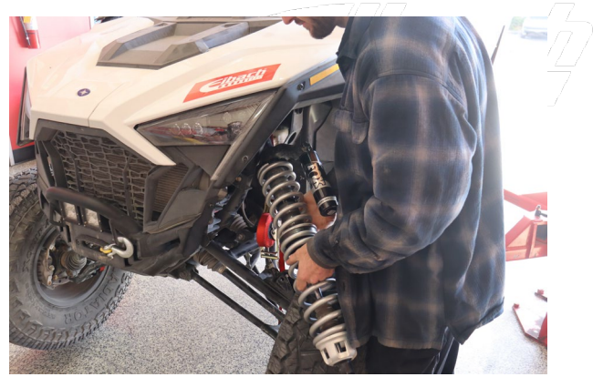
Reinstall the assembled coilover.
