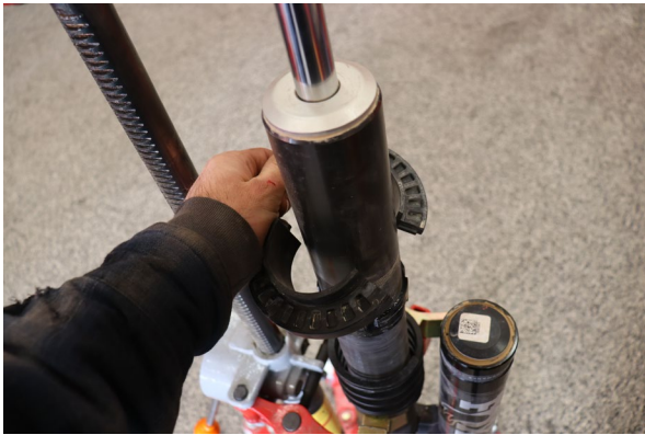
Remove the OE 2-piece secondary slider.
