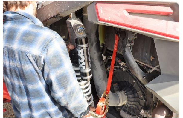
Remove the rear Shock.
