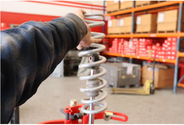
Install the Eibach tender spring.
