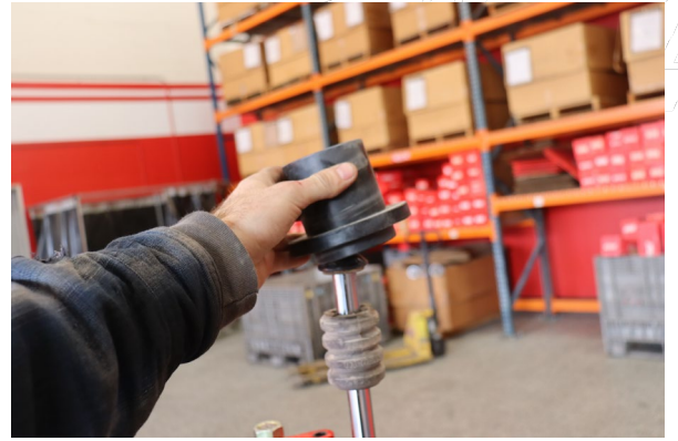
Install the Eibach slider.
