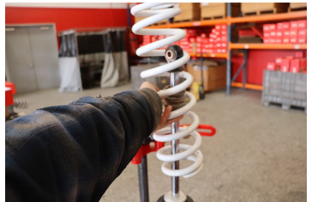
Remove the OE main spring.
