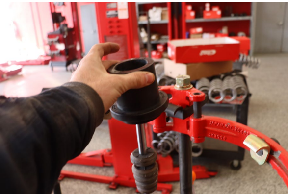
Install the Eibach front slider.
