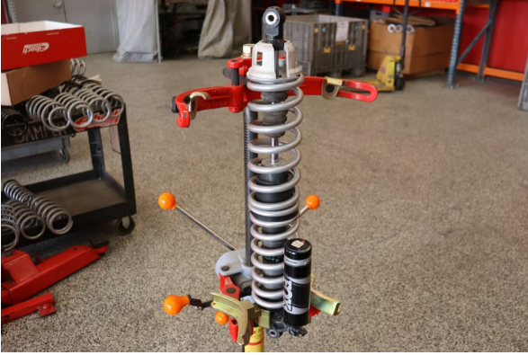
Reinstall the OE spring seat.
