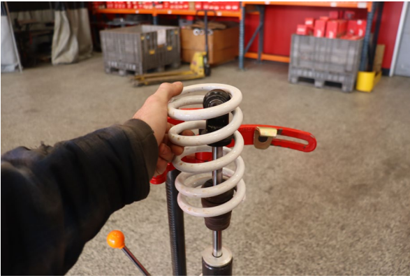
Remove the OE tender spring.
