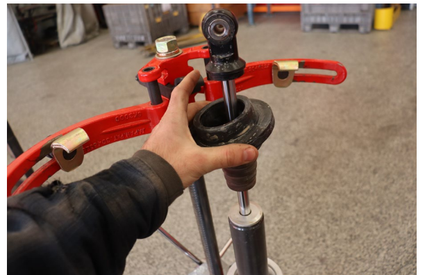
Remove the OE slider.
