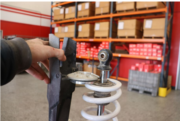
Compress the springs and remove the lower spring perch. Note the orientation of the dust shield relative to the reservoir.
