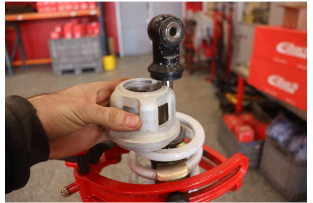
Compress the springs and remove the lower spring perch.
