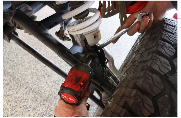
Loosen and remove the upper and lower shock bolts.
