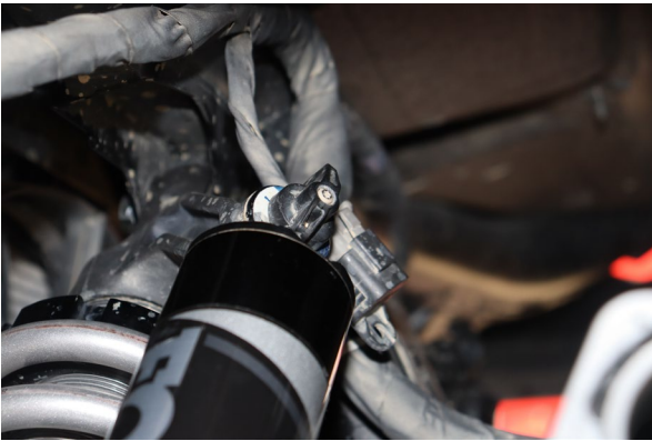
We recommend setting the clicker to position 2 to start.
