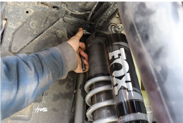
Reinstall the assembled coilover.
