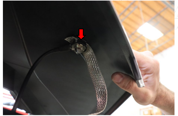
The antenna will need to be removed by removing the hex bolt underneath the hood.
