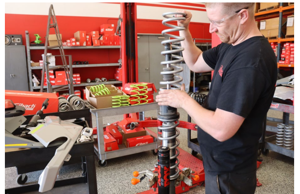
Install the Eibach main spring.
