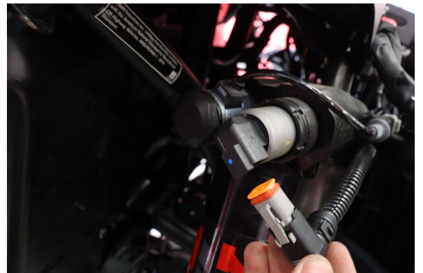
Unplug the Live Valve compression and rebound cables.
