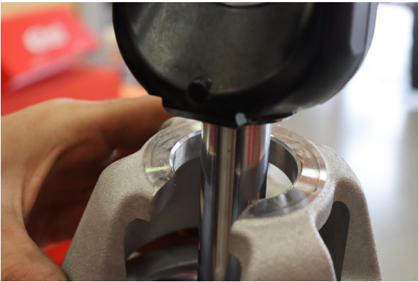
Install the OE lower spring perch. Make sure the perch is lined up with the boss on the clevis as shown.
