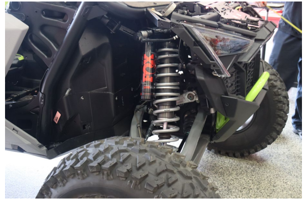
Repeat on the opposite side and reinstall everything in reverse order of removal. Torque shock bolts to factory spec.
