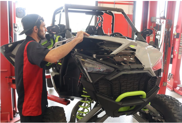
Once everything is removed you can access the shock bolts.
