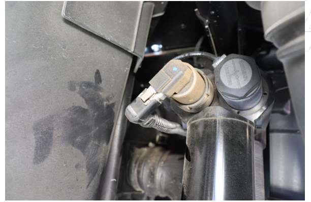
Unplug the harnesses for the Live Valve compression and rebound adjusters.
