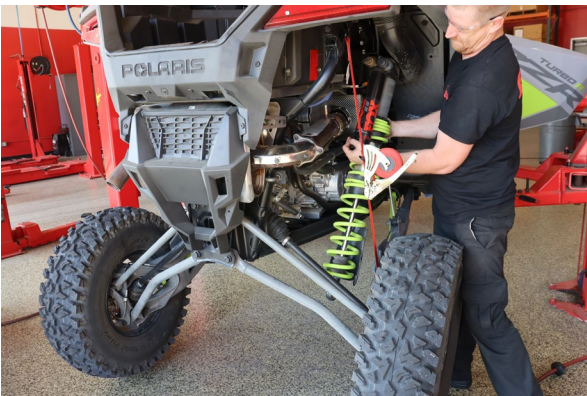
Remove the rear shock assembly.
