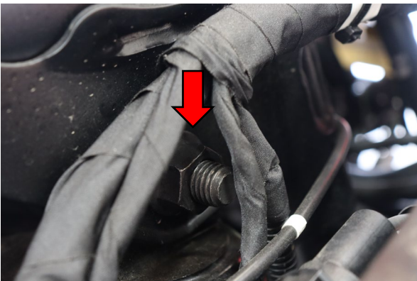
Loosen and remove the upper shock bolt with a 21mm wrench.
