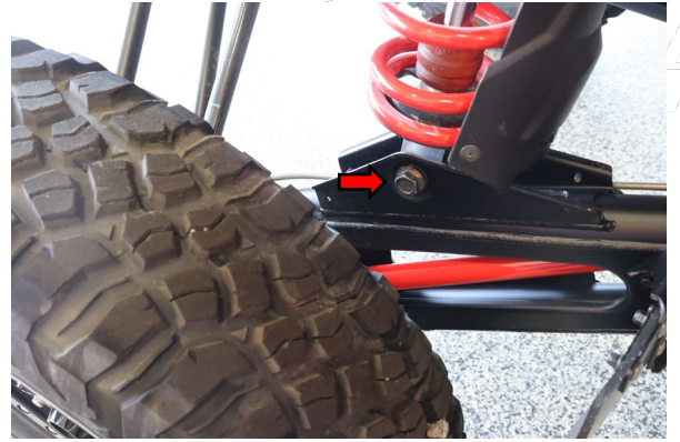
Loosen and remove the lower shock bolt
