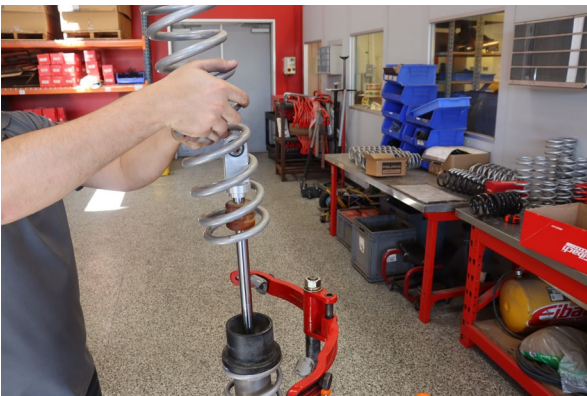
Install the Eibach rear main spring and compress the springs.
