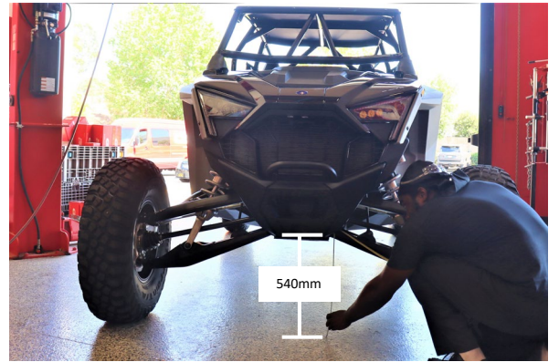
The front height should measure about 540mm from the ground to the lower control arm bolt. The shock eye to eye length should be about 805mm.
