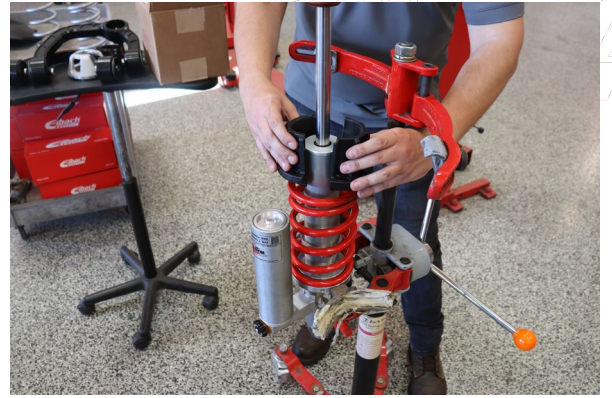
Remove the stock slider.
