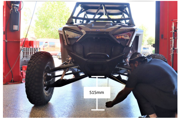
The front height should measure about 515mm from the ground to the lower control arm bolt. The shock eye to eye length should be about 800mm.
