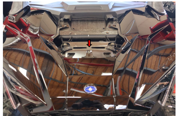
Remove the torx screw securing the front hood fascia. Push it toward the front of the car to release. For vehicles equipped with front camera unplug the harness.
