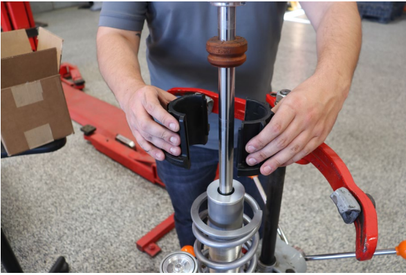
Install the OE 2-piece slider.
