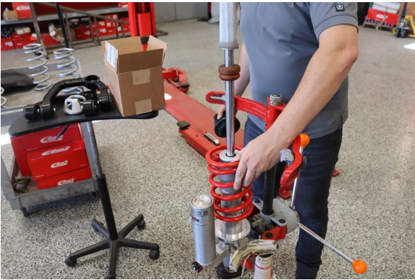
Remove the OE front tender spring.
