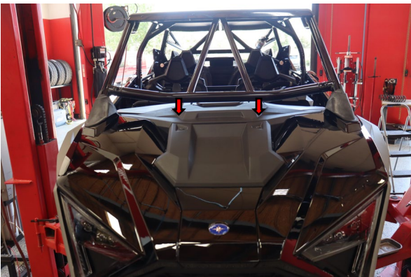
Remove the torx screws with securing the upper hood scoop
