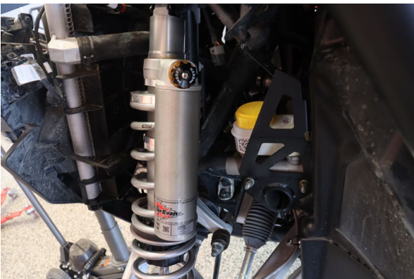
Set the adjuster to 3 clicks clockwise from the full open (soft) position.
