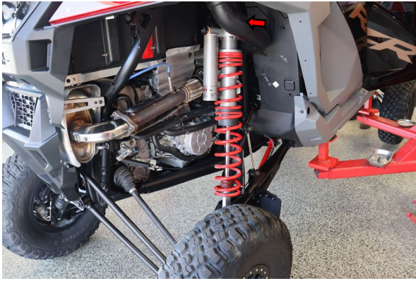
Jack up the rear of the car so the wheels are off the ground. Loosen and remove the upper shock bolt.
