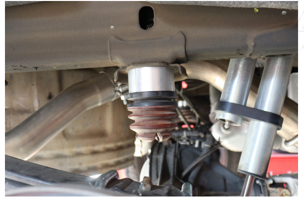
Reinstall with the provided bump stop spacer and bolt.
