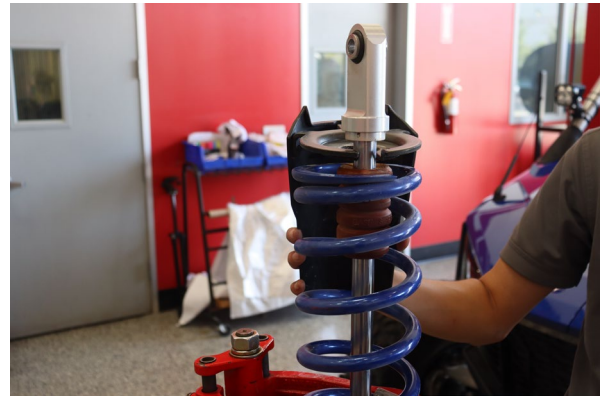
Compress the springs and remove the lower spring perch with the guard attached.
