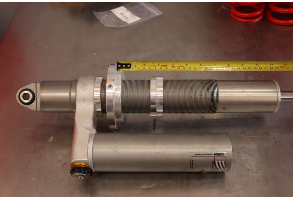
Set the crossover ring to 85mm front the spring seat to the bottom of the crossover ring.
