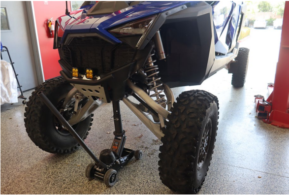
Begin by jacking up the front of the vehicle.
