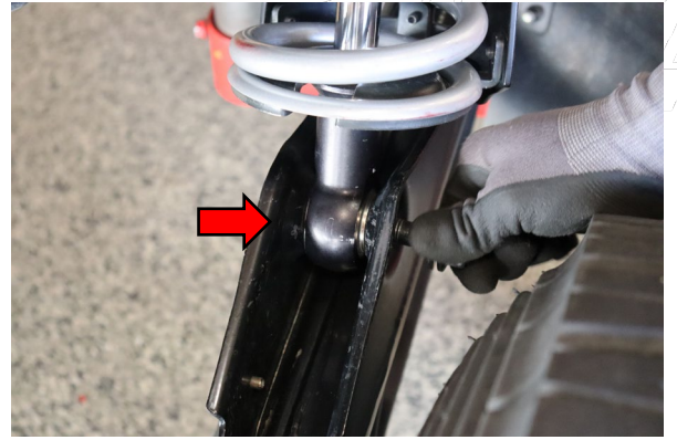
Remove the lower shock bolt with a 21mm socket.
