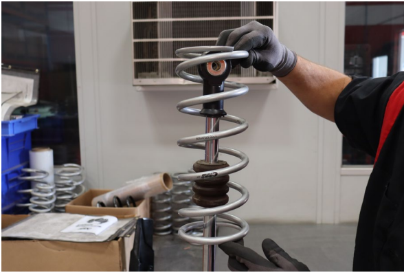
Install the Eibach secondary spring.
