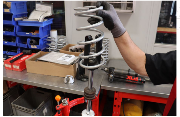
Install the Eibach secondary spring.
