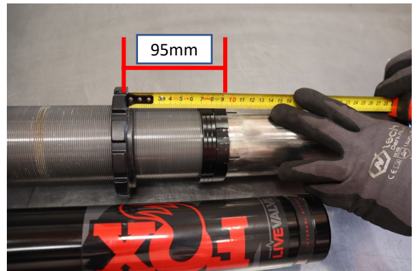
Set the crossover ring to 95mm from the bottom of the spring seat to the bottom of the crossover rings.
