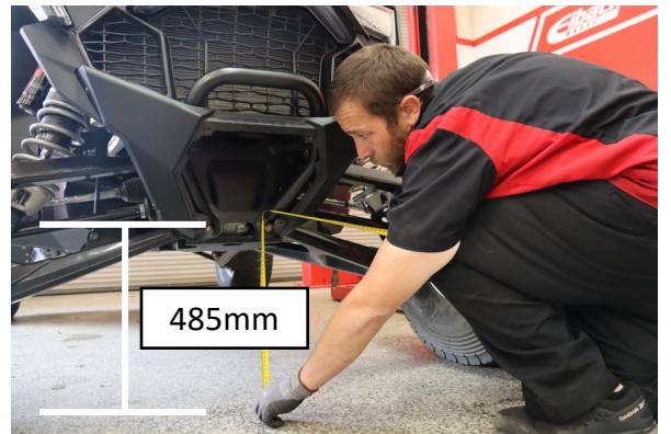
Measure from the ground to the center of the lower control arm bolt. The recommended preload measurement above should get close to the recommend ride height of about 485mm
