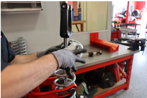
Make sure the OE spring retainer is fully seated with the notch matching the lower clevis.
