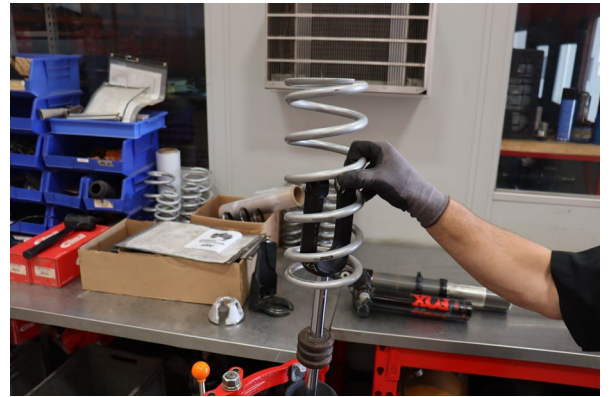
Install Eibach main spring
