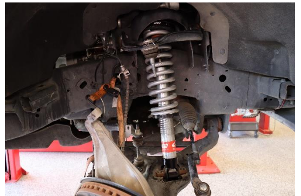
Step 11. Install new Eibach Coilover shocks
