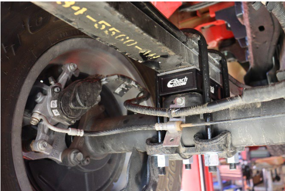
9a. Reinstall the OE U-bolt bracket. Secure the bracket with the provided washers and nuts. Tighten the nut with a 22mm wrench. Then to torque the U-Bolt nuts to 100 ft-lbs. Do not over tighten.
