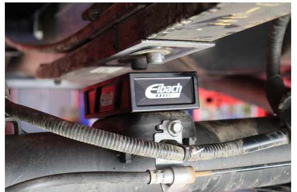
Install the new Eibach lift block.
