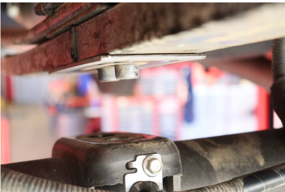
Lower the axle. Make sure any brake lines or wires do not overstretch when lowering the axle.
