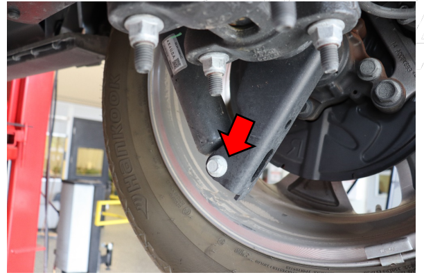
Loosen and remove the lower shock bolt.
