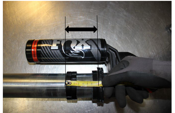
Step 10. Install the cross-over rings and set them at 75mm measuring from the spring flange to the bottom of the crossover ring.
