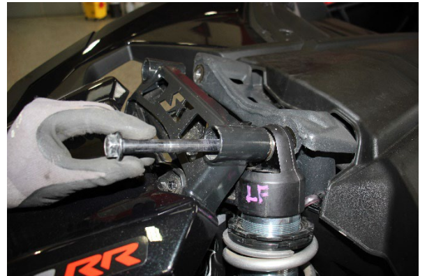
Step 16. Secure the coilover to the upper mount with the OE hardware, leaving loose for now.
