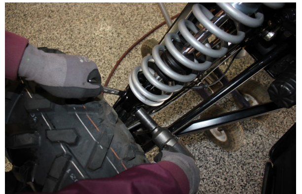
Step 18. Secure the coilover to the control arm with the OE hardware. Tighten the upper mount hardware.
