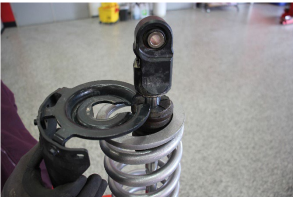
Step 17. Compress spring assembly and re-install spring retainer. Note: The spring seat is shaped to locate and go on only one way, ensure it is installed with the flat on the seat lined up with the flat on the rod end.
