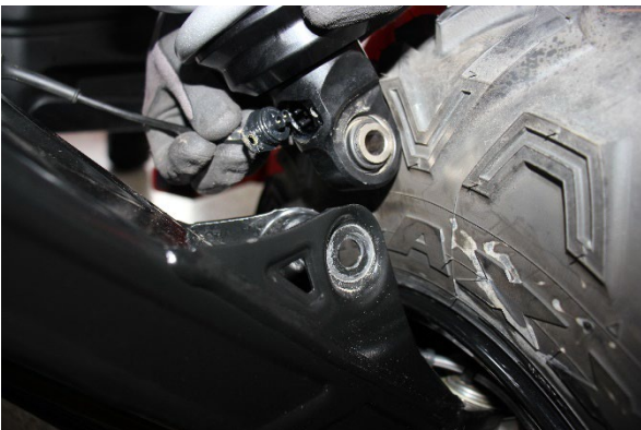
Step 17. Carefully plug the electrical connector back in at the bottom of the coilover, secure with OE allen screws. Note: There is a locator pin on the connector, ensure it is clocked properly. Do not over tighten connector.
