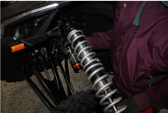
Step 15. Re-install the coilover.
