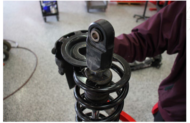
Step 8. Compress the OE spring assembly and remove the spring retainer. Note: The bump stop will need to be pried down, out of the way of the spring retainer.
