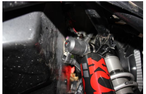
Step 18. Plug in the electrical connector at the top of the coilover.
