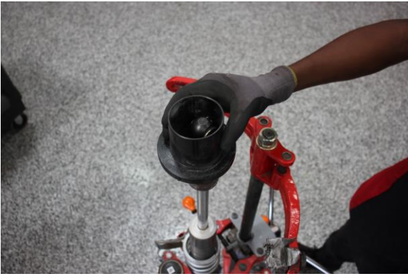
Step 7. Remove OE spring slider.
