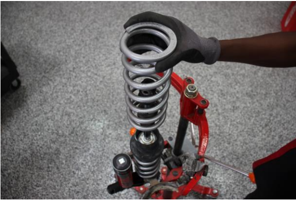
Step 13. Install the Eibach main spring.
