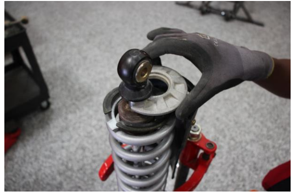
Step 14. Compress the spring assembly and re-install the spring retainer and rock guard.
