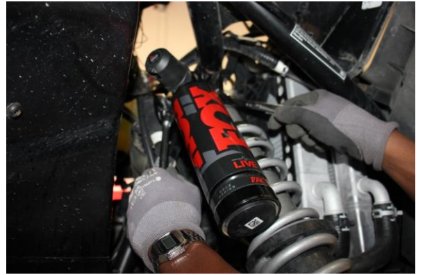
Step 16. Secure the coilover to the upper mount with the OE hardware.
