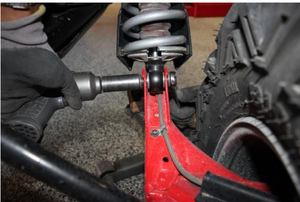
Step 17. Secure the coilover to the control arm with the OE hardware.
