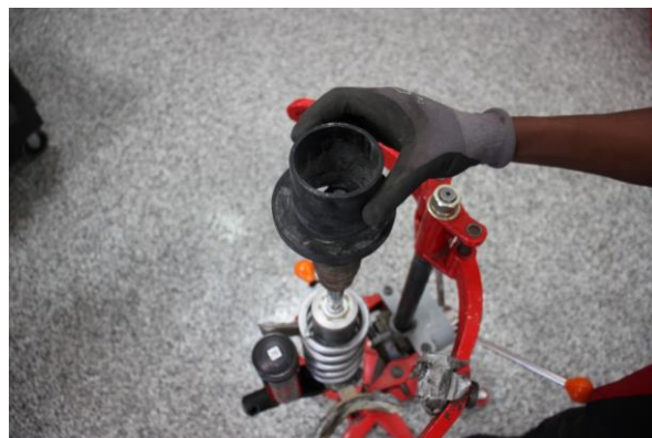
Step 12. Install the Eibach spring slider.
