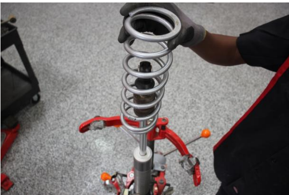
Step 11. Install the Eibach secondary spring.
