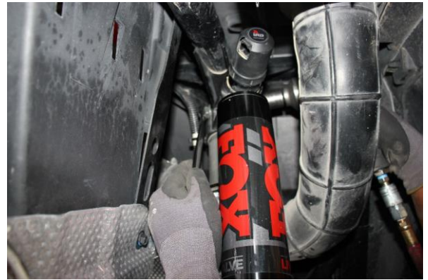
Step 16. Secure the coilover to the upper mount with the OE hardware.
