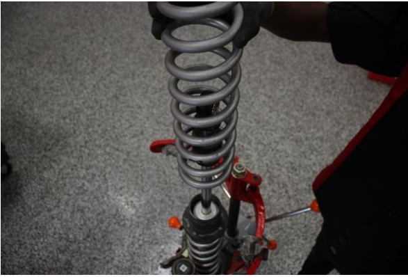
Step 13. Install the Eibach main spring.
