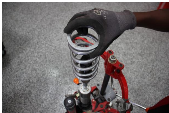
Step 11. Install the Eibach secondary spring.
