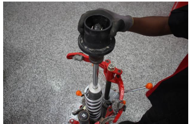
Step 12. Install the Eibach spring slider.
