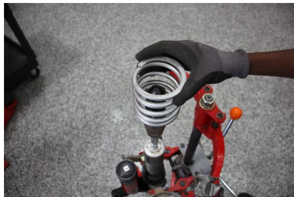
Step 8. Remove OE secondary spring.
