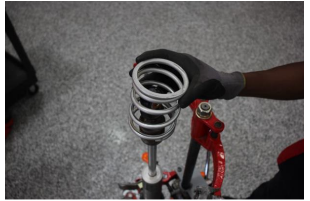
Step 8. Remove OE secondary spring.
