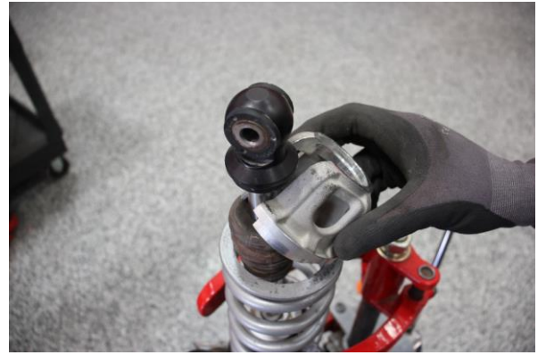
Step 14. Compress the spring assembly and re-install the spring retainer.
