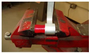
2. Insert supplied crush sleeves into the hourglass bushings.
