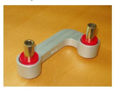
3. Install the new end links and the new sway bar in reveres order of removal using the new supplied hardware.
