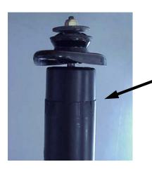
You must remove the rear shock, then, remove the upper mount to access the rear bump stop which is located underneath the OE dust boot
